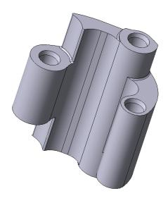
Experience with mass production of similar components has shown how porosity could become an extremely critical aspect due to metal shrinkage in feeder proximity where the material solidifies later and contracts while cooling. The simulation analysis focuses mainly on the solidifying phase, with the objective of finding a configuration that allows homogeneous cooling of the part avoiding the creation of hot areas.
